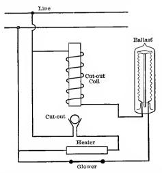
FIG. 157. Diagram of circuits in the Nernst lamp.
